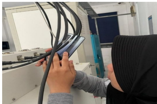
Figure 2. NFC Tag Scanning Process Using a Smartphone
